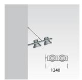
Wall-mounted linear structure for installation of 2 medium-sized body Maxiwoody projectors without bracket
