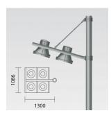
Single square structure for installation of 4 medium-sized body Maxiwoody projectors with bracket
