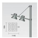
Single square structure for installation of 4 small-body Maxiwoody projectors with bracket
