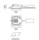
Sistema Easy FL - Recessed fitting complete with inductive control gear with inverter 2x18 W TC-DEL
