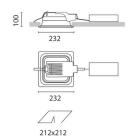
Sistema Easy FL - Recessed fitting complete with digital dimmable electronic (DALI) control gear 42 W TC-TEL (HIGH EFFICIENCY FIXTURE)
