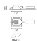
Sistema Easy FL - Recessed fitting complete with digital dimmable electronic (DALI) control gear 2x26 W TC-DEL (HIGH EFFICIENCY FIXTURE)
