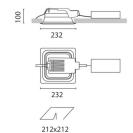
Sistema Easy FL - Recessed fitting complete with analogue dimmable electronic (1-10V) control gear 2x32 W TC-TEL Attention! Code out of production - 2012
