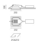
Sistema Easy FL - Recessed fitting complete with electronic control gear 2x32 W TC-TEL
