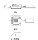
Sistema Easy FL - Recessed fitting complete with electronic control gear 2x26 W TC-DEL
