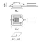
Sistema Easy FL - Recessed fitting complete with electronic control gear 2x18 W TC-DEL
