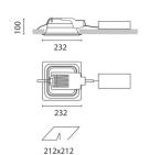
Sistema Easy FL - Recessed fitting complete with electronic control gear 26 W TC-DEL
