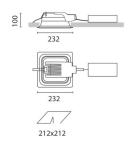
Sistema Easy FL - Recessed fitting complete with electronic control gear 18 W TC-DEL
