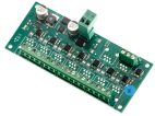
Code: 187 DMX splitter Electronic device to regenerate the DMX signal. 1 input and 7 output. 12÷24Vdc Power supply to be ordered (87 or 175 recommended)
