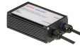
Code: 141 Supported n. of lamps: 10 Power supply with DMX interface for RGB fixtures 36W/220÷240V-3CHx350mA (3CHx10x1W) DMX control allowed IP67 CLASS I SELV EQ.
