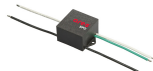
Code: 237 SPD: (Surge Protection Device) 275Vac Maximum discharge current 10KA (8/20 \mu s) Maximum operating current 5A Suitable for series connection - IP66
