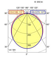
Light sourceLEDWork equipmentWithoutConnected load22 - 26 V; DCPower consumptionca. 26 WLuminous fluxapprox. 650 lmLuminous efficiencyapprox. 23 lm/W
