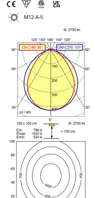
Light source LED Work equipment Without **Connected load** 22 - 26 V; DC **Power consumption** ca. 21 W Luminous flux approx. 2.750 lm Luminous efficiency approx. 130 lm/W Light type/-color Cold white Colour temperatur approx. 5.000 K Color rendering index CRI ≥ 80 Light distribution Direct Beam angle 85° / 101° **Chromaticity tolerance LED** < 4 SDCM Glare control Screen System of protection IP 54 Class of protection
