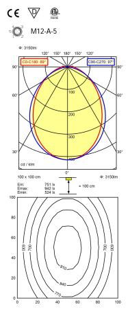
light source LED work equipment without connected load 22-26 V, DC env. 25 W power consumption luminous flux approx. 3.150 lm luminous efficiency approx. 126 lm/W light type/-color cold white colour temperatur approx. 5.000 K CRI > 80 color rendering index light distribution direct beam angle 89° / 97° chromaticity tolerance LED < 4 SDCM glare control screen system of protection IP 54 class of protection
