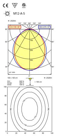
light source LED work equipment without connected load 22-26 V, DC env. 20 W power consumption luminous flux approx. 2.520 lm luminous efficiency approx. 126 lm/W light type/-color cold white colour temperatur approx. 5.000 K CRI > 80 color rendering index light distribution direct beam angle 89° / 97° chromaticity tolerance LED < 4 SDCM glare control screen system of protection IP 54 class of protection
