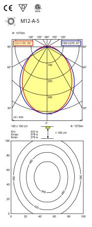
light source LED work equipment without connected load 22-26 V, DC env. 12,5 W power consumption luminous flux approx. 1.575 lm luminous efficiency approx. 126 lm/W light type/-color cold white colour temperatur approx. 5.000 K CRI > 80 color rendering index light distribution direct beam angle 89° / 97° chromaticity tolerance LED < 4 SDCM glare control screen system of protection IP 54 class of protection
