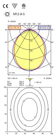
Light source LED Work equipment Without Connected load 22 - 26 V; DC ca. 24 W **Power consumption** Luminous flux approx. 2.520 lm Cold white Light type/-color Colour temperatur approx. 5.000 K Color rendering index CRI ≥ 80 Direct **Light distribution** 89° / 97° Beam angle **Chromaticity tolerance LED** < 4 SDCM Glare control Screen System of protection IP 54
