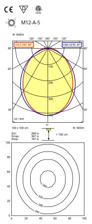
Light source LED Work equipment Without Connected load 22 - 26 V; DC ca. 9 W **Power consumption** approx. 945 lm Luminous flux Cold white Light type/-color Colour temperatur approx. 5.000 K Color rendering index CRI ≥ 80 **Light distribution** Direct 89° / 97° Beam angle **Chromaticity tolerance LED** < 4 SDCM
