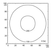
Light source LED Work equipment Without 16 - 32 V; DC **Connected load Power consumption** ca. 10 W approx. 950 lm Luminous flux Light type/-color Daylight Colour temperatur approx. 5.400 K Color rendering index CRI ≥ 80 **Light distribution** Direct **Direct ratio** approx. 82 % Beam angle >120° **Chromaticity tolerance LED** < 5 SDCM Glare control Without Luminance (L65)  $\leq 8.000 \text{ cd/m}^2$ Unified glare rating (4H 8H) ≤ 25
