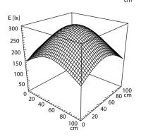
Light source LED Work equipment Without 20 - 28 V; DC **Connected load Power consumption** ca. 12 W Luminous flux approx. 800 lm Light type/-color Cold white Colour temperatur approx. 5.000 K Color rendering index CRI ≥ 80
