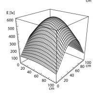
Light source LED Work equipment Without 20 - 28 V; DC **Connected load Power consumption** ca. 12 W Luminous flux approx. 820 lm Light type/-color Cold white Colour temperatur approx. 5.000 K Color rendering index CRI ≥ 80
