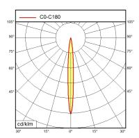
Light sourceLEDWork equipmentWithoutConnected load24 V; AC; DCPower consumptionca. 6 WLuminous fluxapprox. 400 lmLight type/-colorDaylightColour temperaturapprox. 5.400 K
