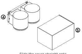
Slide the cover straight onto the device (not skewed) to prevent the springs from deforming
