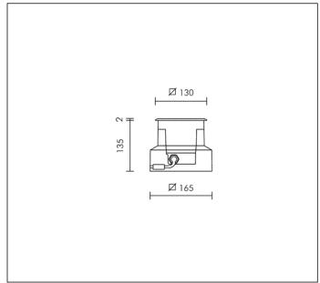
3 MODULES LED RGB 24V PWM Rated luminaire luminous flux: 53lm
