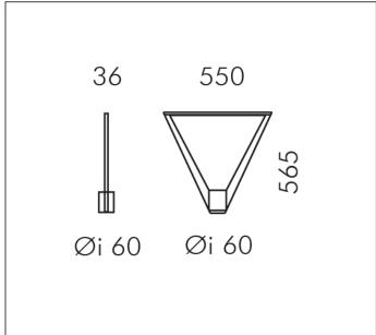
MODULES LED 4000K 230V 3360lm CRI 80 Rated luminaire luminous flux: 1721lm
