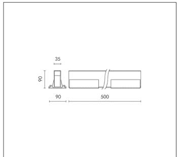
MODULES LED 4000K 24V 389Im CRI 80 Rated luminaire luminous flux: 178lm
