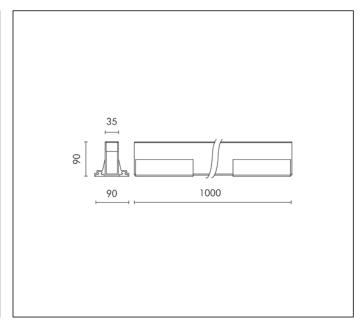
MODULES LED 3000K 24V 740lm CRI 80 Rated luminaire luminous flux: 330lm
