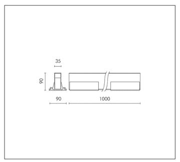
MODULES LED 3000K 24V 740lm CRI 80 Rated luminaire luminous flux: 202lm
