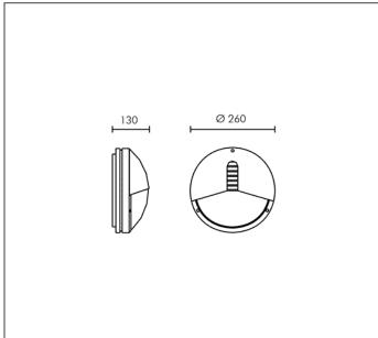
TC-DEL 18W G24q-2 1200lm Rated luminaire luminous flux: 372lm
