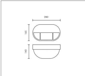
TC-DEL 18W G24q-2 1200lm Rated luminaire luminous flux: 288lm
