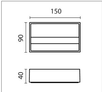
MODULES LED 4000K 230V 428lm CRI 70 Rated luminaire luminous flux: 211lm
