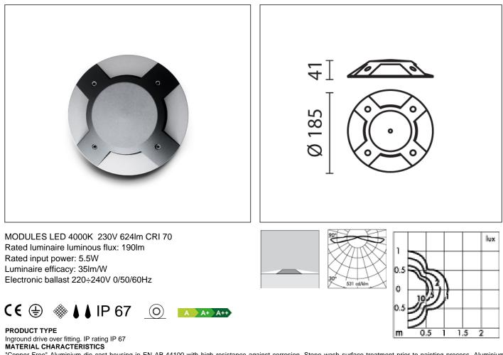
"Copper Free" Aluminium die cast housing in EN AB-44100 with high resistance against corrosion. Stone wash surface treatment prior to painting process. Aluminium protective guard of 8 mm thickness.A4 grade Stainless Steel screws with 2,5-3% molybdenum content which increases the resistance against corrosion. Pre treated Silicone Gaskets. Painting Process : 3 Step Process
