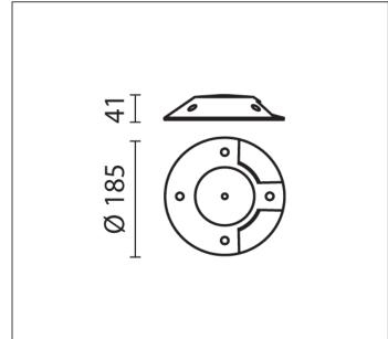
MODULES LED 3000K 230V CRI 80 Rated luminaire luminous flux: 76lm Rated input power: 4.3W
