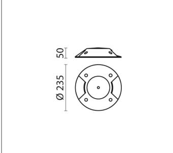
MODULES LED 4000K 230V 566lm CRI 70 Rated luminaire luminous flux: 209lm
