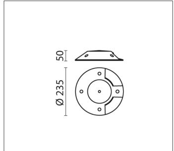
MODULES LED 3000K 230V CRI 80 Rated luminaire luminous flux: 131lm
