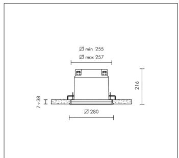
HIT-CRI 35W CLEAR G12 3300lm Rated luminaire luminous flux: 1943lm
