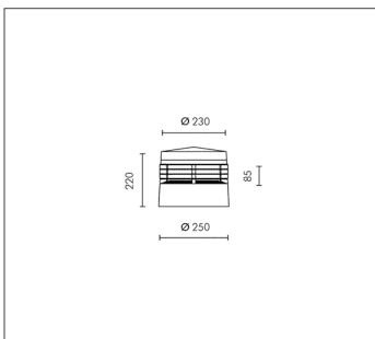
HIT-CRI 70W CLEAR G12 6600lm Rated luminaire luminous flux: 1914lm
