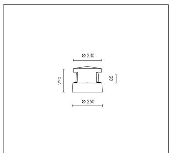
TC-TEL 26W Gx24d-3 1800lm Rated luminaire luminous flux: 198lm
