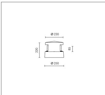
HIT-CRI 70W CLEAR G12 6600lm Rated luminaire luminous flux: 1452lm
