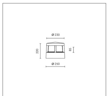
TC-TEL 26W Gx24d-3 1800lm Rated luminaire luminous flux: 414lm
