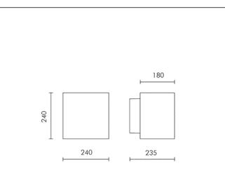
HIT-CRI 70W CLEAR G12 6600lm Rated luminaire luminous flux: 2706lm Rated input power: 84W Luminaire efficacy: 32lm/W (LOR: 42%) Magnetic trasformer 230÷240V 50Hz EEI=A3, LOSSES=12.2W
