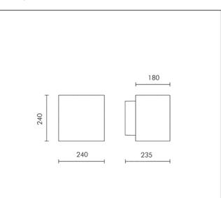
HIT-CRI 70W CLEAR G12 6600Im Rated luminaire luminous flux: 1122Im Rated input power: 84W Luminaire efficacy: 13Im/W (LOR: 18%) Magnetic trasformer 230÷240V 50Hz EEI=A3, LOSSES=12.2W
