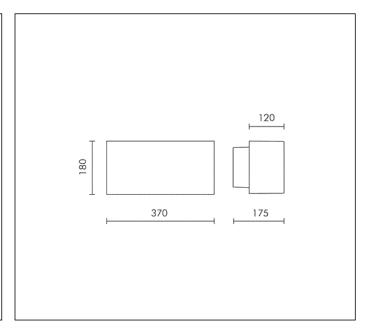
MODULES LED 4000K 4018lm CRI 90 Rated luminaire luminous flux: 2508lm
