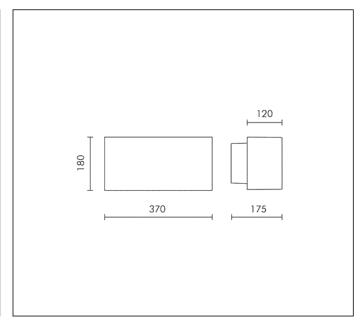
2x TC-D 18W G24d-2 1200lm Rated luminaire luminous flux: 360lm
