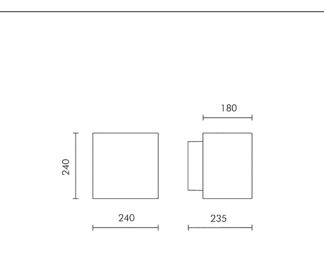
HIT-CRI 70W CLEAR G12 6600lm Rated luminaire luminous flux: 1320lm Rated input power: 84W Luminaire efficacy: 16lm/W (LOR: 8%) Magnetic trasformer 230÷240V 50Hz EEI=A3, LOSSES=12.2W
