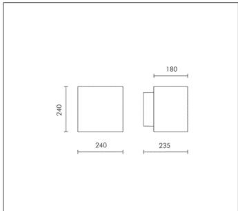
HIT-CRI 70W CLEAR G12 6600lm Rated luminaire luminous flux: 660lm
