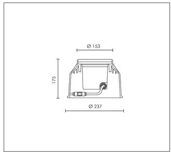
MODULES LED RGB 24V PWM Rated luminaire luminous flux: 19lm
